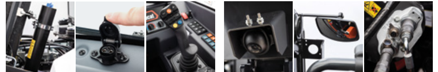
Boom suspension (Nitrogen accumulator) Tractor socket (12 V, 15 A) Smart joystick with Boom float and bucket shaking Rear view camera Rear mirror Built-in electric socket (2 lines)
