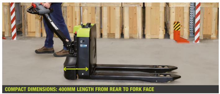
The WPio15 is a versatile pallet truck with a load capacity of 1.5 tons which is suitable for various tasks in daily material transport. The vehicle is equipped with an integrated charger as standard and can be charged at any 230 volt socket. Thanks to the spring-loaded lateral support rollers, the vehicle has excellent driving behaviour in curves which ensures safe and efficient transport of goods.
